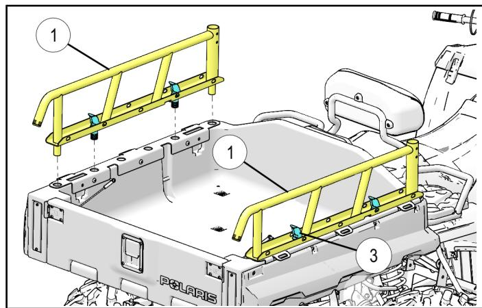
4. Rotate LOCK & RIDE® upper cams (3) as shown to lock in place. If installation is loose, unlatch cam, rotate clockwise to tighten, and re-latch.
