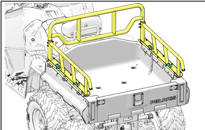
7. Yukon adventure rack kit can be removed by unlocking the LOCK & RIDE® expansion anchors ③. Lift rack kit assembly away from the vehicle bed as shown.
