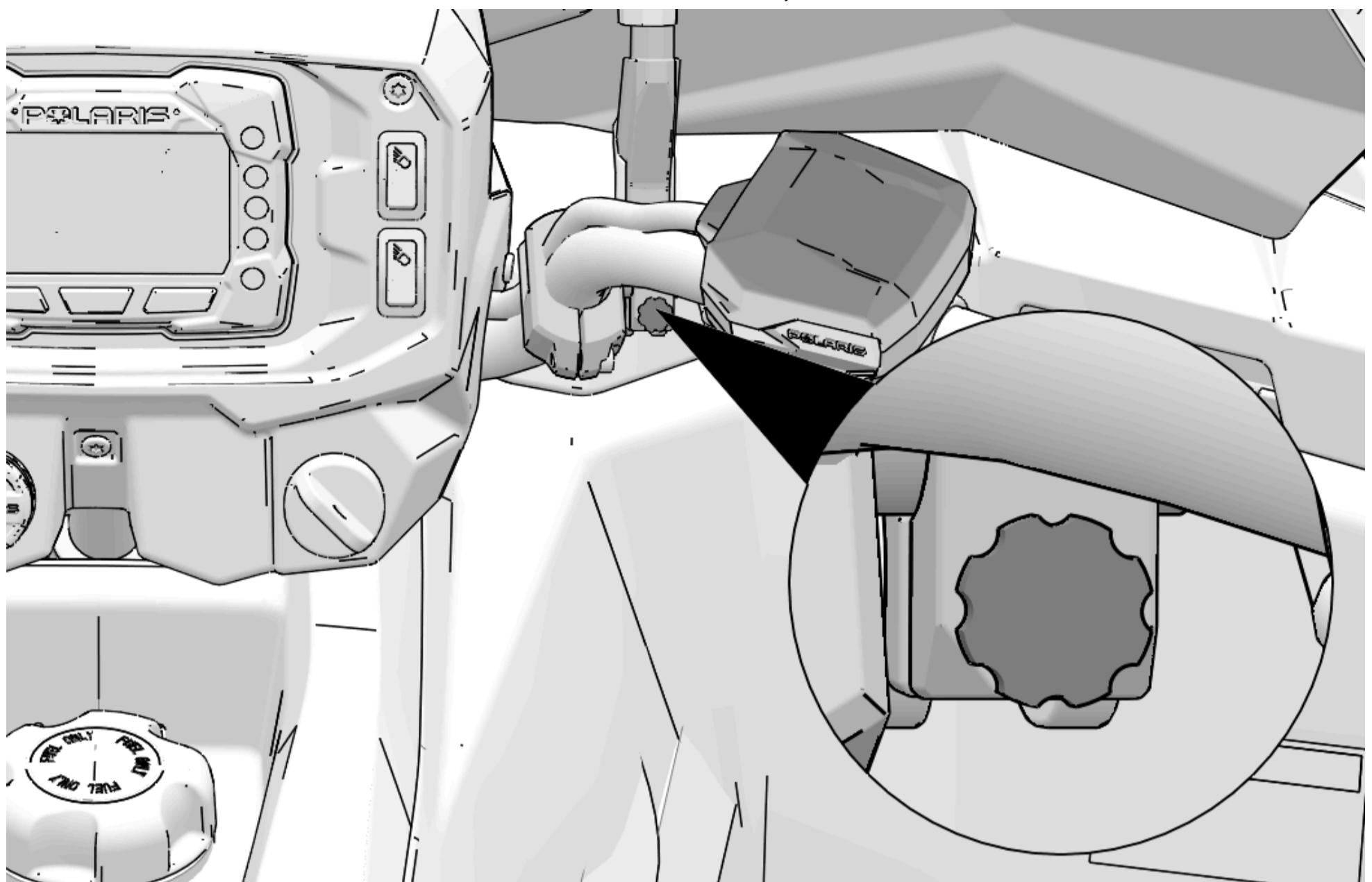
2. Remove mount covers and loosen fasteners on the inside of the windshield to adjust windshield position. Adjust as needed and torque fasteners to specification. Reinstall the mount covers.
