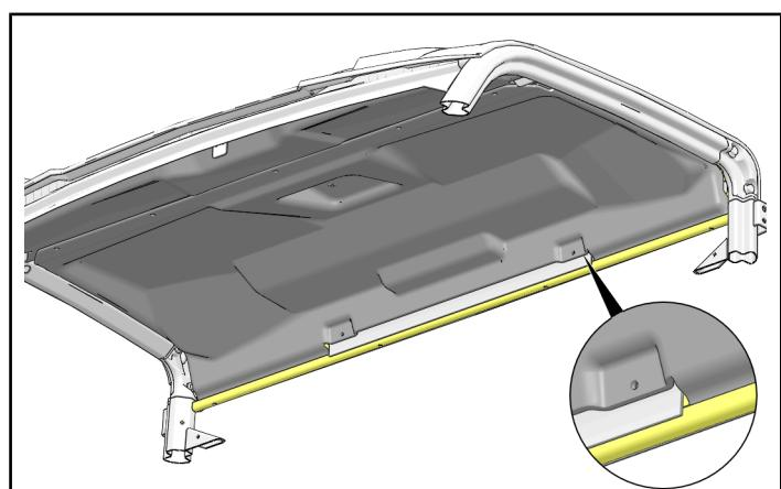
4. If installing optional light, then refer to instructions included with light. Otherwise, install two each screws ④ and washers ③ through rear liner ② into roof.
