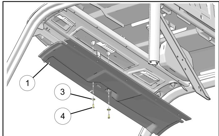
3. Insert both rear segments ④ of rear liner ② into roof support channel, then slowly tip liner up, inserting left and right edges of liner between ROPS and roof seal.
