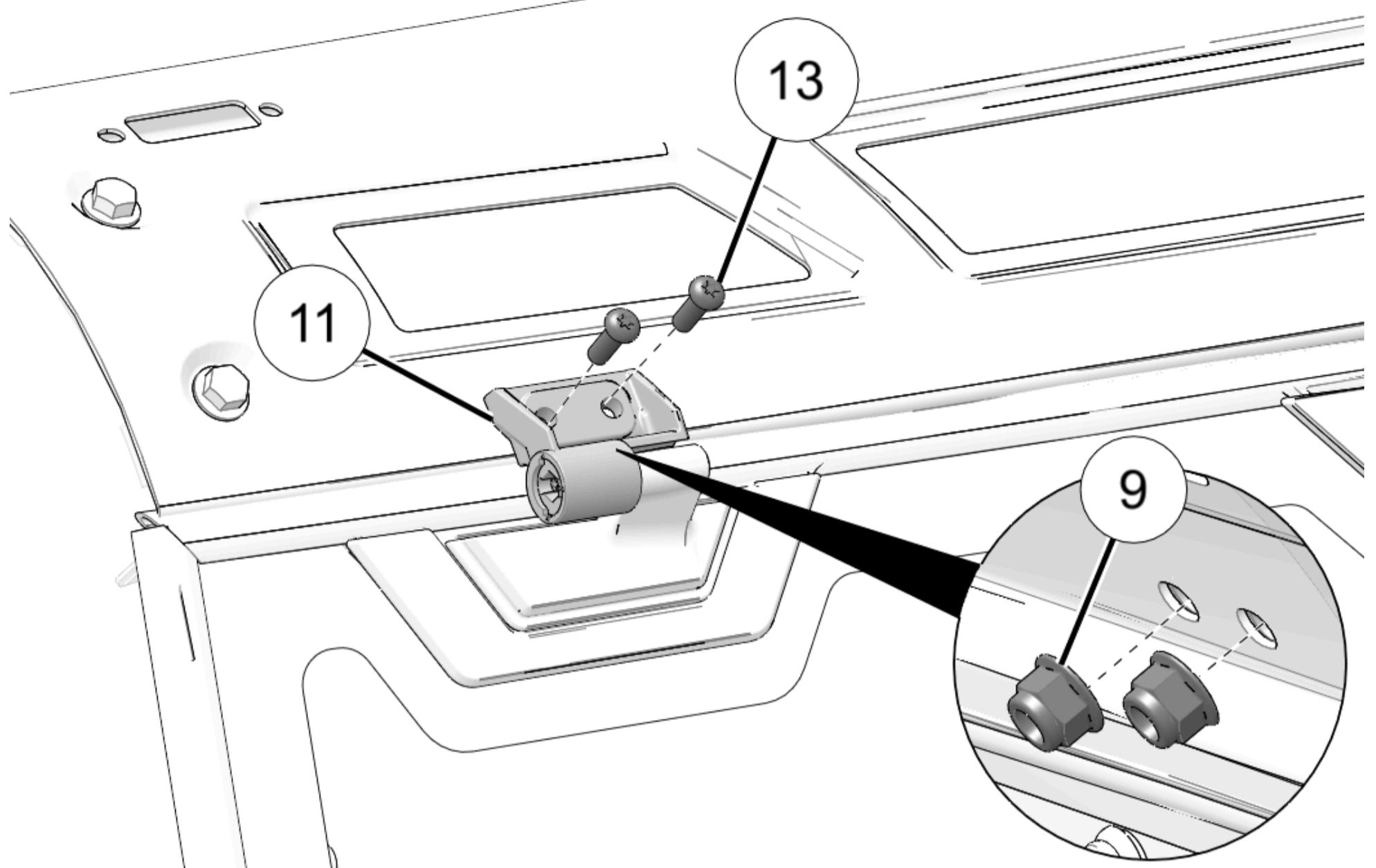
6. Torque two left side and two right side windshield mount nuts (9) to specification.
