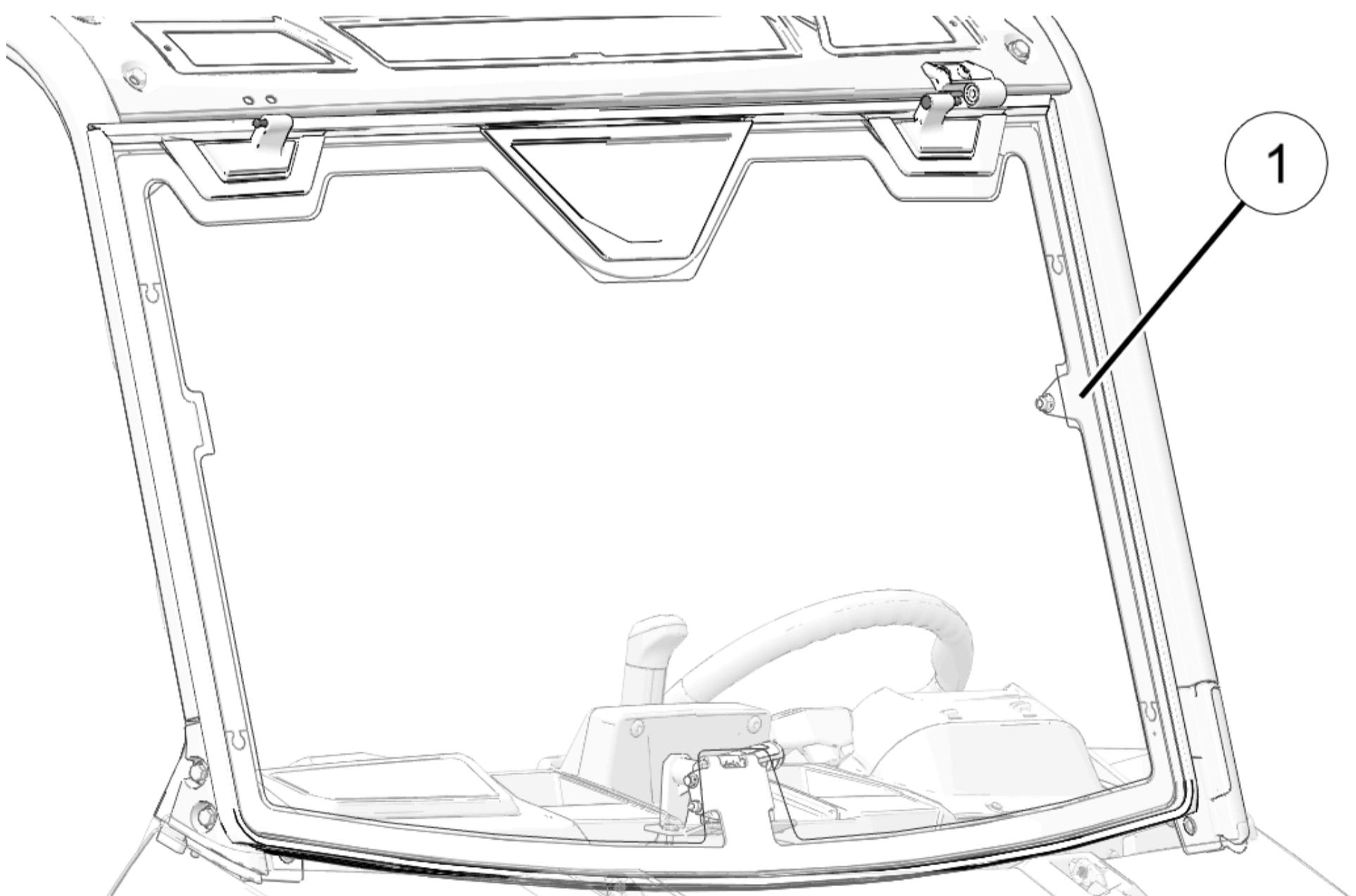
3. Move pin on left side windshield hinge into bushing on left side windshield mount ⑫.
