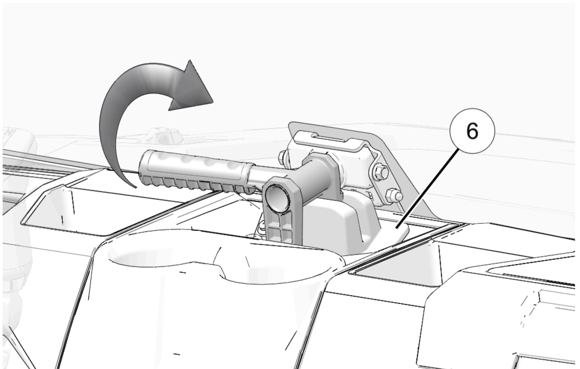
2. Move windshield handle forward and align handle legs over handle base (6) in the vented position, as shown.
