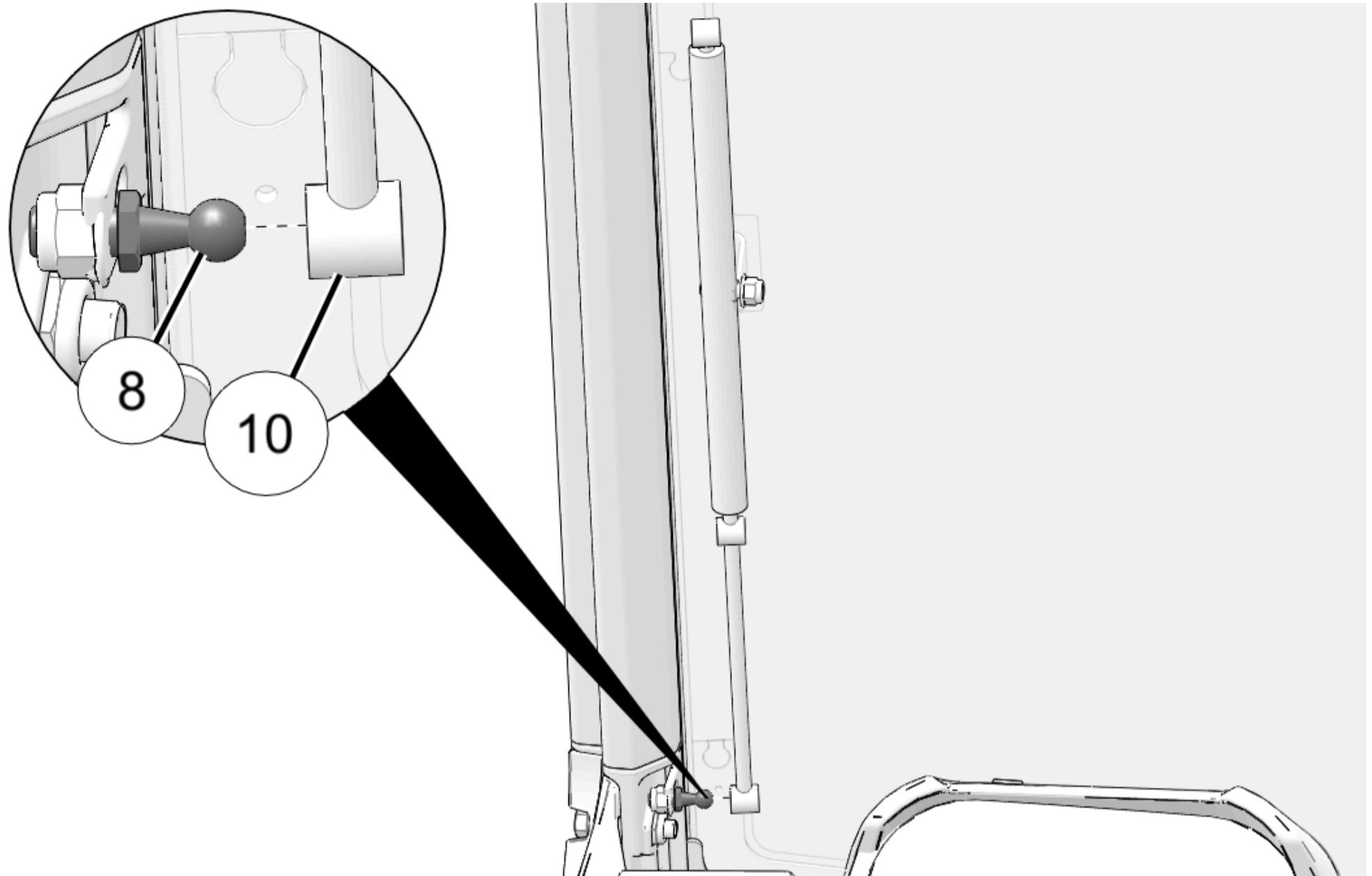
4. Open windshield and push upper shock cylinder **10** into upper ball fitting **8**.
