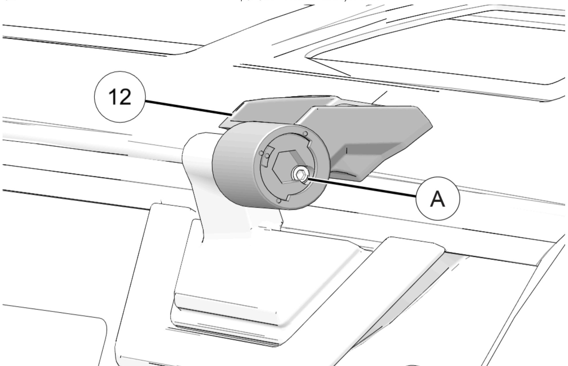
2. Turn hinge pin cam **B** in either direction to center the windshield on the vehicle.
