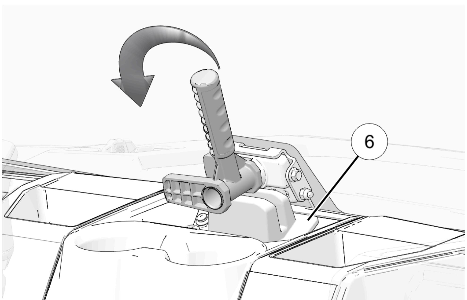
3. Make sure windshield seals are compressed and that the windshield opens and closes correctly. See Windshield Alignment section if adjustments are needed.
