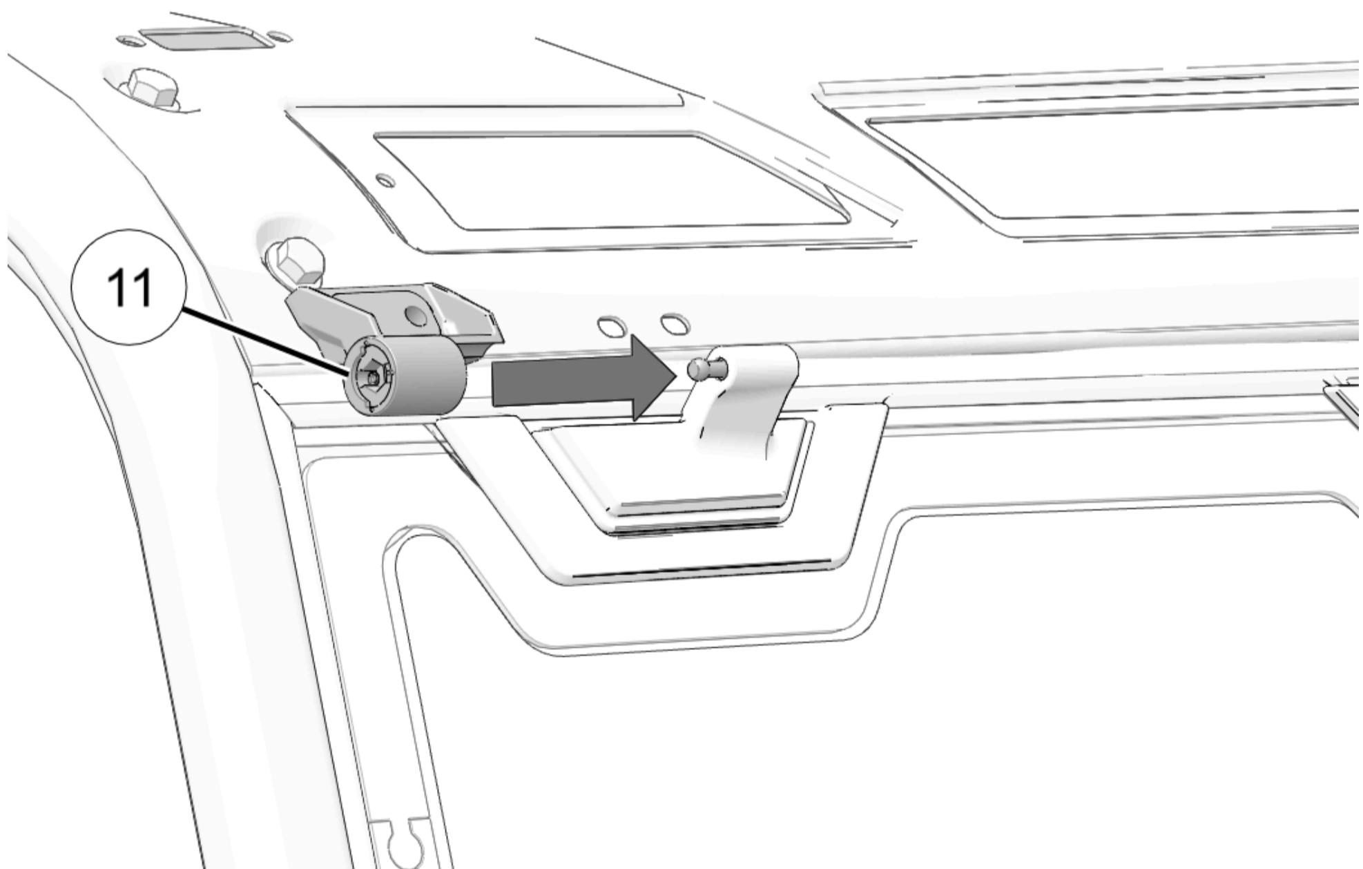
5. Install right side windshield mount (11) to upper ROPS with two screws (13) and two nuts (9).
