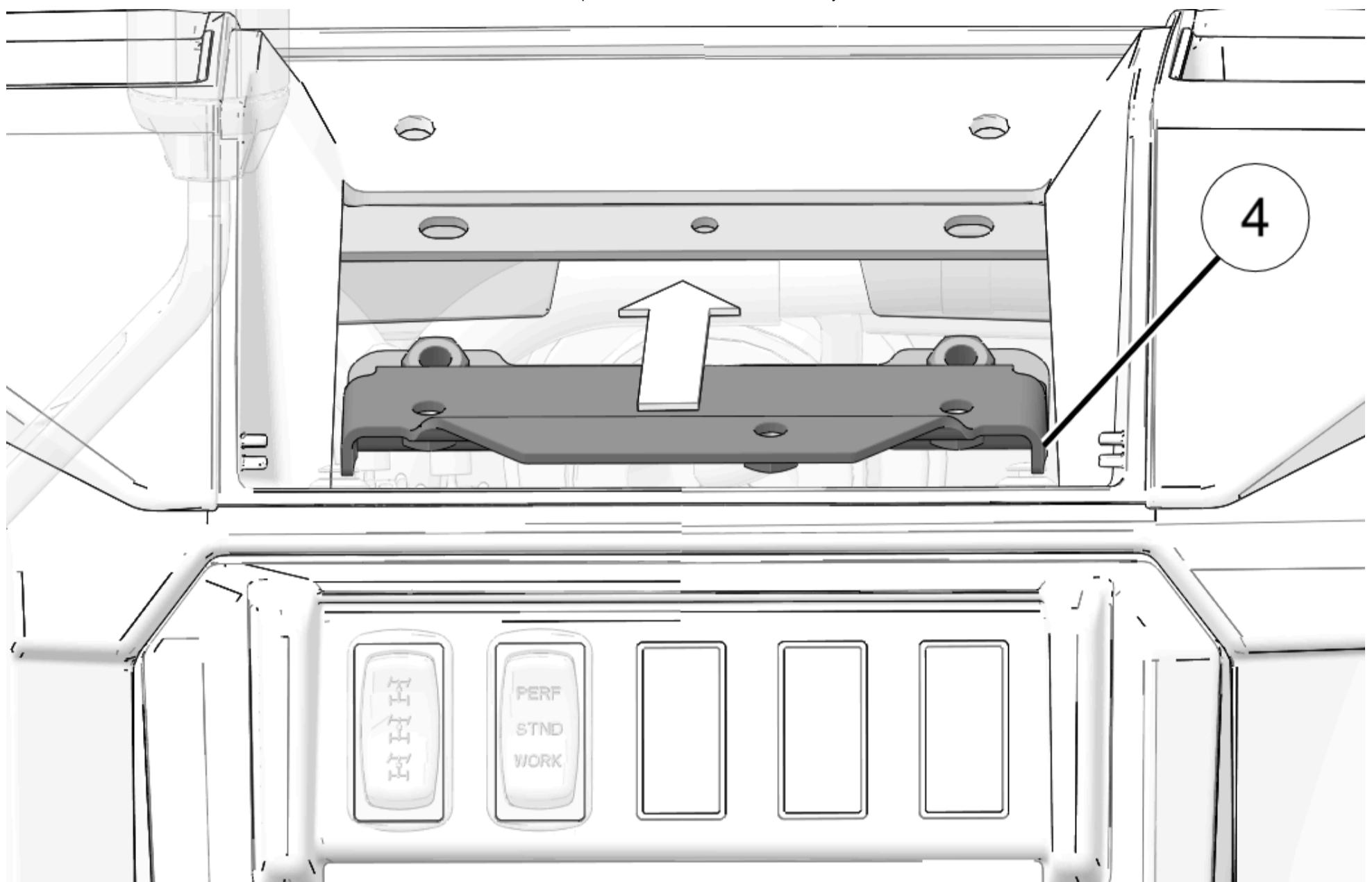
2. Install backer bracket (4) to upper chassis bar with two screws (5).
