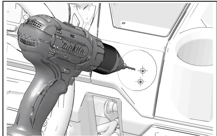
4. Install holder ⑯ to dash with two screws ⑯. Tighten screws until fully seated.
