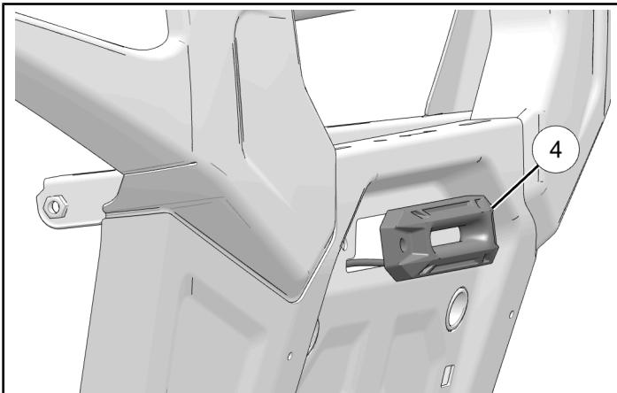
2. Loosely install two screws ② through upper holes on winch into vehicle front support structure.
