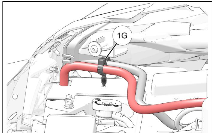
8. Route chassis harness through harness routing tab on winch bracket.
