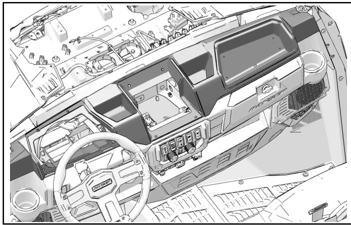
2. Install autostop fairlead ④ and fairlead backer plate ③ to bumper using two screws ⑤.
