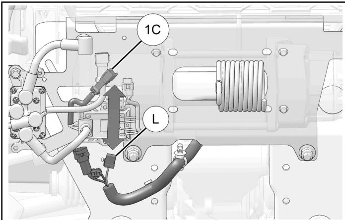
10. Install fir tree clip on chassis harness to winch bracket.
