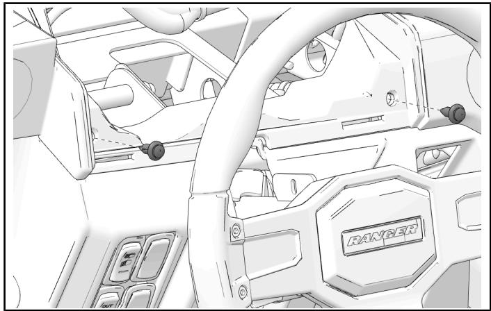
6. Remove and keep six screws from front of upper dash.
