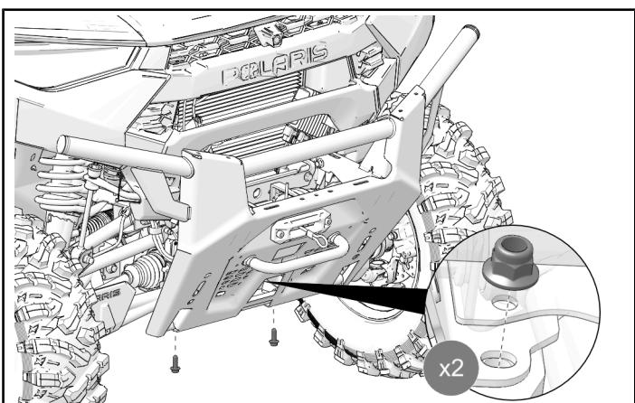
4. Torque fasteners to specification.
