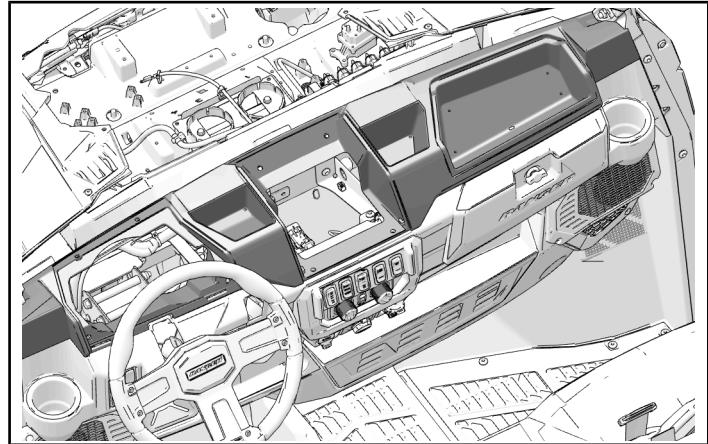
2. Install using six kept screws onto front of upper dash. Tighten screws until fully seated.
