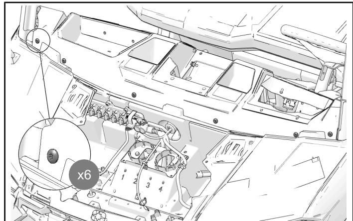
3. Install two kept push-pin rivets in instrument cluster area.
