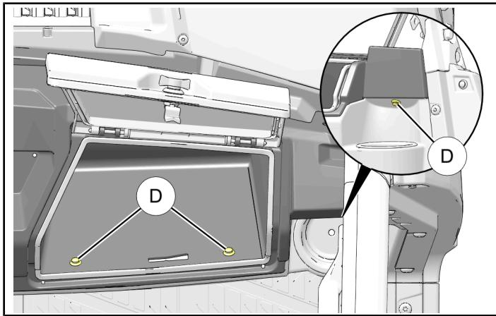
5. Move upper dash (with instrument cluster) backwards, then disconnect instrument cluster wiring harness.
