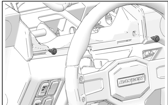
4. Install two kept push-pin rivets in center cup holder area.
