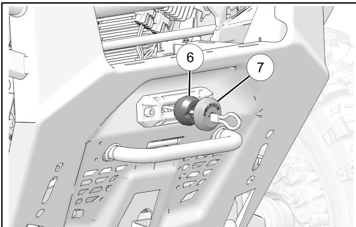
2. Install hook **⑧** to loop at end of rope with clevis and cotter pin. Make sure cotter pin is secured.
