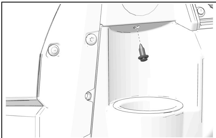
2. Remove and keep one push-pin rivet from top of passenger side cup holder.
