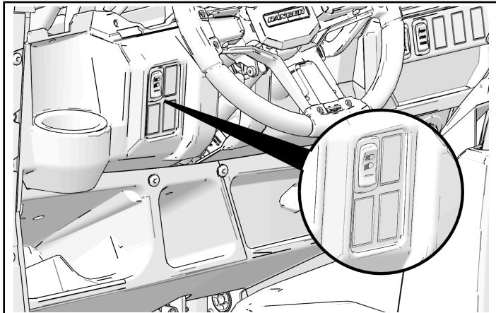
3. Pull the jumper harness connector ⑫ through the dash cutout and connect to the winch switch ⑪. Make sure the connector is fully seated into the switch.
