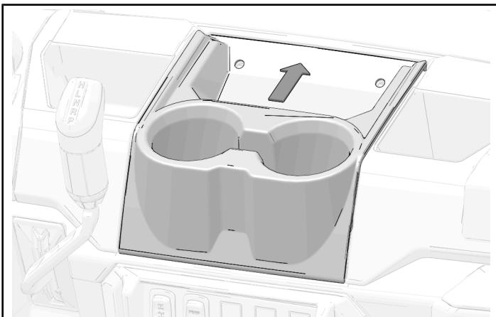
2. Install the instrument cluster bezel with two kept push-pin rivets.
