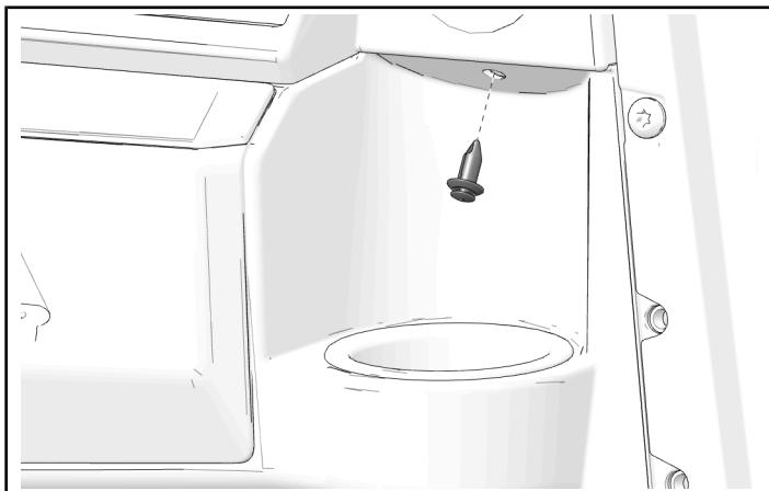
3. Remove and keep two push-pin rivets from upper storage compartment area.
