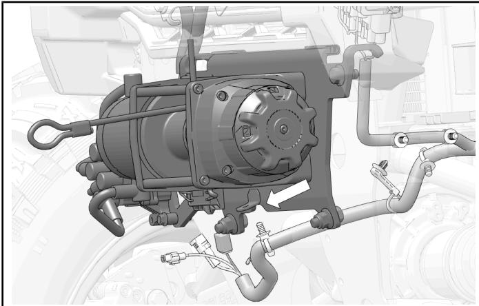
9. Remove and discard cap from chassis harness connector **L**. Connect winch connector **1C** to chassis harness connector **L**.
