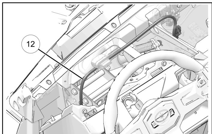
6. Install jumper harness ⑫ to connector 14C located on the wireless receiver harness ⑭.
