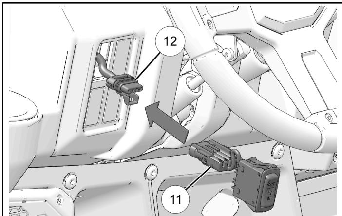
4. Push the switch into the dash cutout until fully seated with an audible click.
