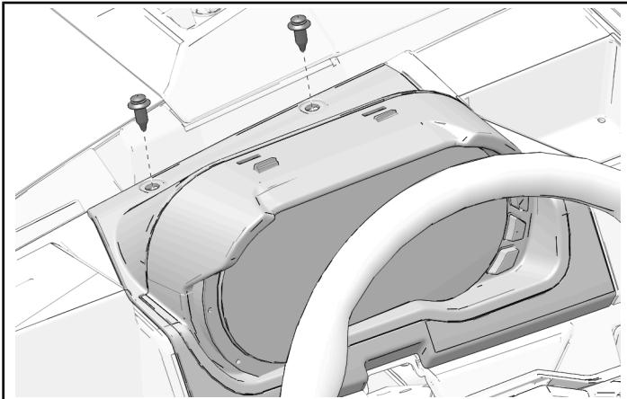
3. Remove the instrument cluster by pulling straight out towards the steering wheel.
