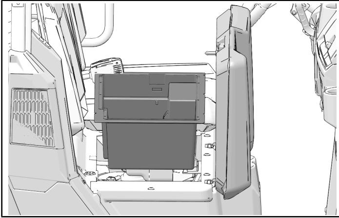
3. Loosen nut on negative (-) wire and remove wire from battery.
