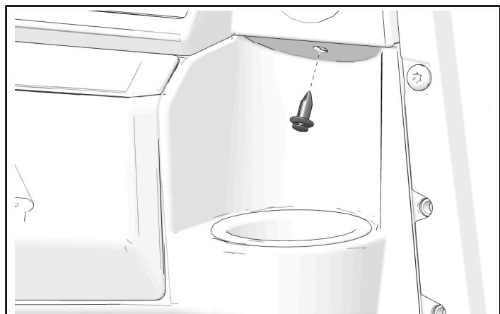
5. Install two kept push-pin rivets in upper storage compartment area.
