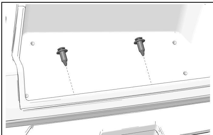
4. Remove and keep two push-pin rivets from center cup holder.
