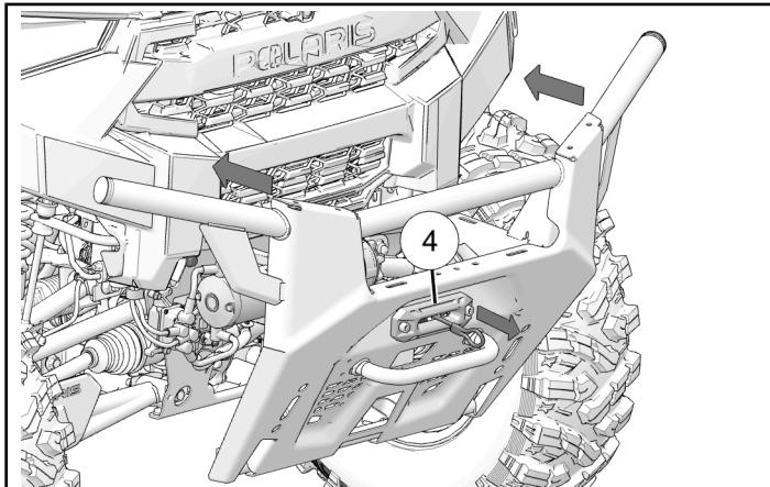
3. Loosely install bottom of bumper to vehicle frame using two kept screws and nuts.
