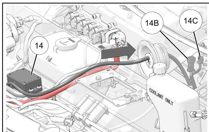
13. Remove and discard cap from winch connector on vehicle harness **M**. Connect wireless receiver connector **14B** to winch connector **M**.
