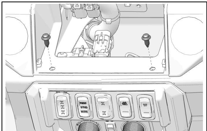
5. Remove and keep two push-pin rivets from instrument cluster.
