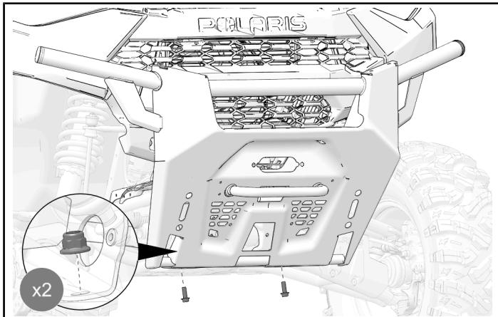
2. Remove and keep two nuts and two screws from front bumper support bracket.
