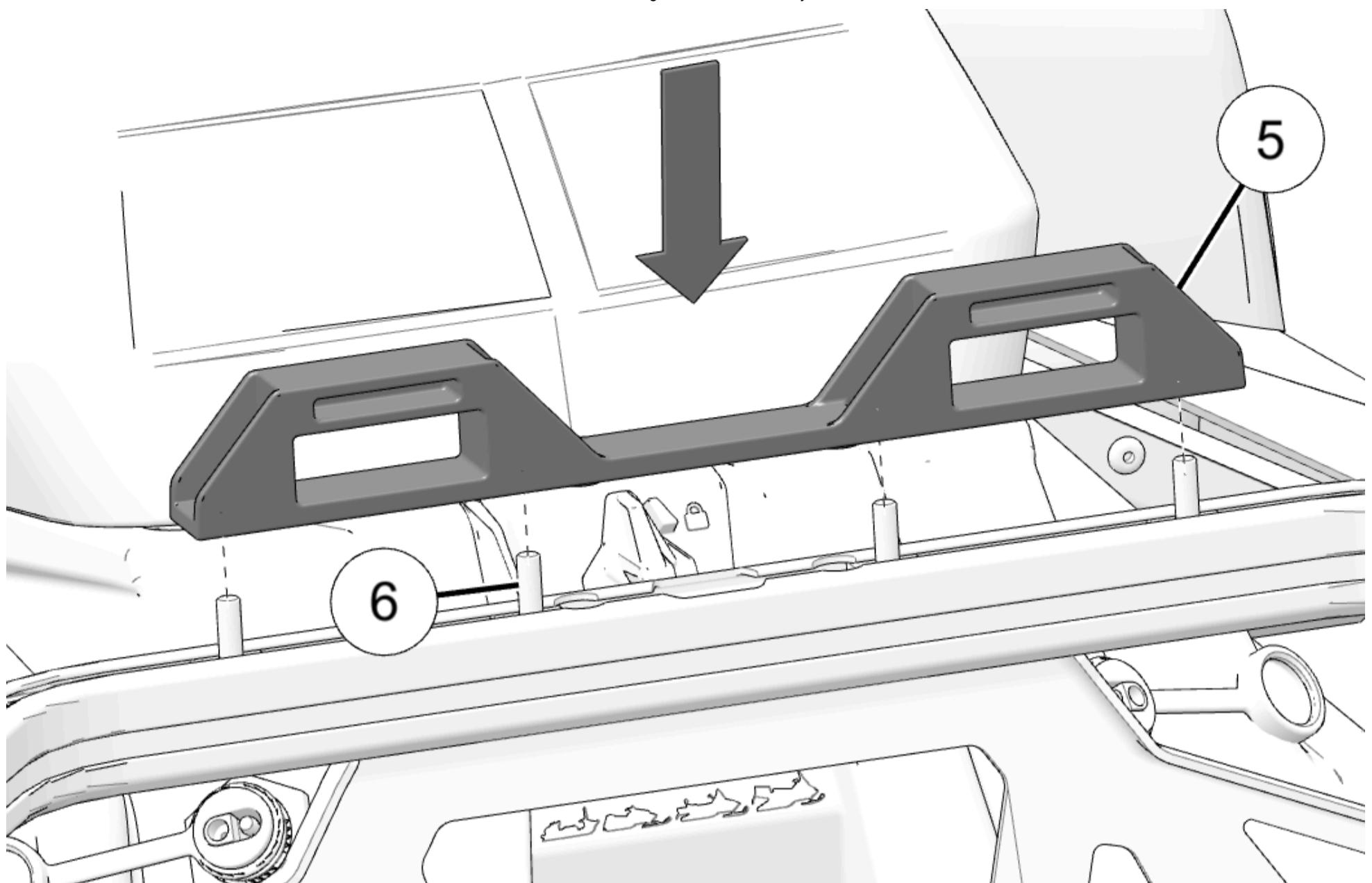
3. Install four nuts **7** to seat support **5**. Torque nuts to specification.
