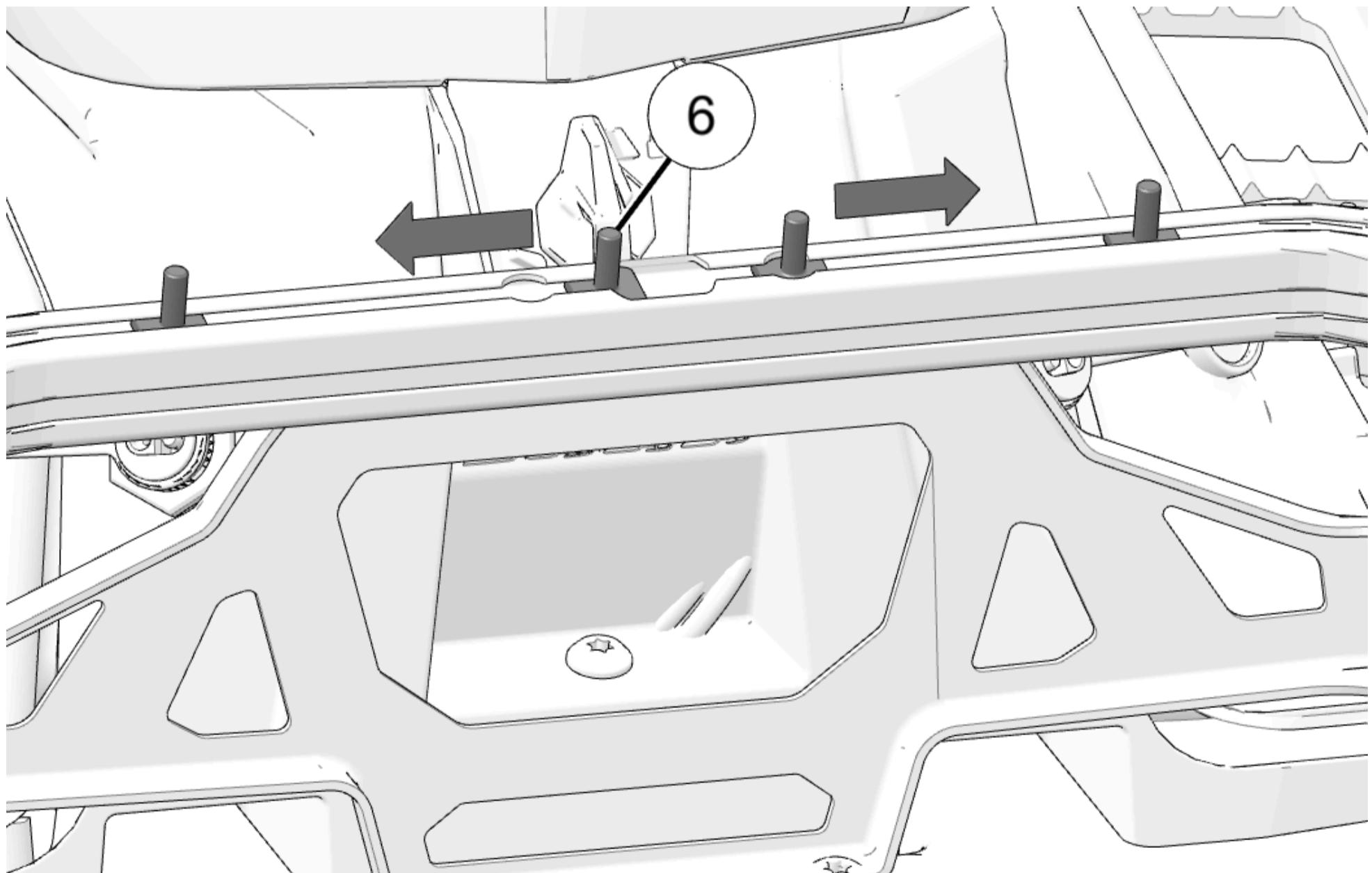
2. Install Lock & Ride Flex® seat support (5) on cargo rack using four screws (6). Make sure screws are aligned with holes in seat support.
